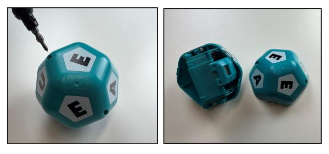
2. Use the screwdriver to remove the battery compartment cover.
