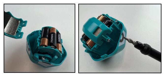
4. Close the device using the curved button notch on the edge as a guide. Do not overtighten the screws.
